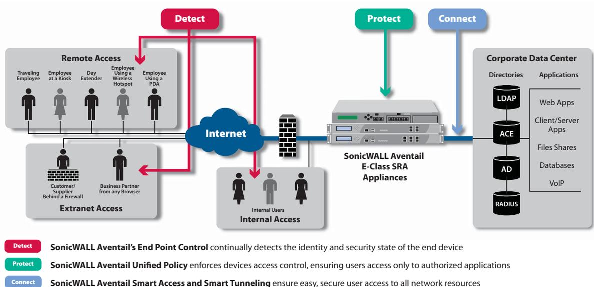
SonicWALL Aventail E-Class Remote Access Solution provides secure access for all users, devices and applications.
